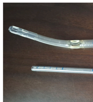
Fig 5 Bottom: Arterial cannula; Top: Venous cannula; Narrow lumen, high pressures in arterial cannula and critical anatomical location (aorta) are contributing factors to technical difficulties when removing arterial cannula.
