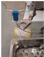
Fig 2. Tubing heated within water bath is less efficient, requires more MDT collaboration.
