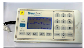
Fig 7 Haemochron Activated Clotting Time (ACT) machine: Used as a clinical tool to overcome anaesthetic bleeding post CPB due to excessive anticoagulant heparin. Achieved via titration of anticoagulant, heparin vs pro-coagulant, protamine.
